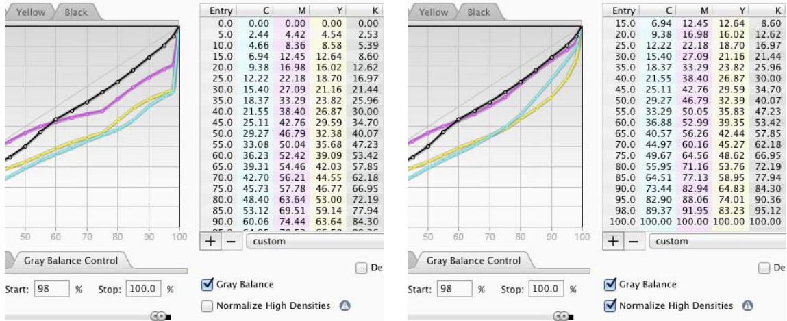
Conventional G7 calibration curves (left) vs. curves with Normalize High Densities ON (right)
