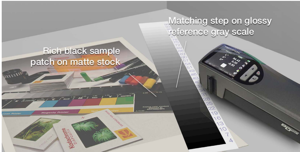
Finding matching neutral densities by eye in a viewing booth.
