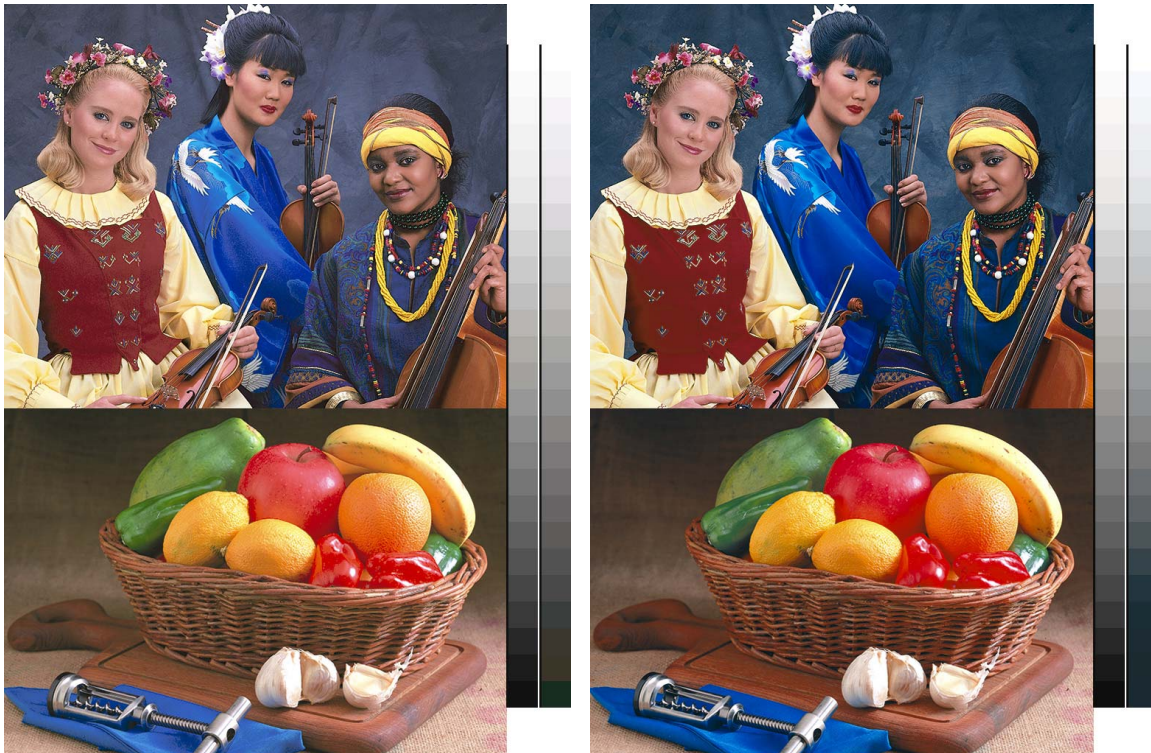
(Left): A high-density ink jet with conventional G7 calibration. (Right): The same printer calibrated with Normalize High Densities. Notice the smoother tonality in high-saturation areas (apple, garments, etc.) in the right-hand sample.
