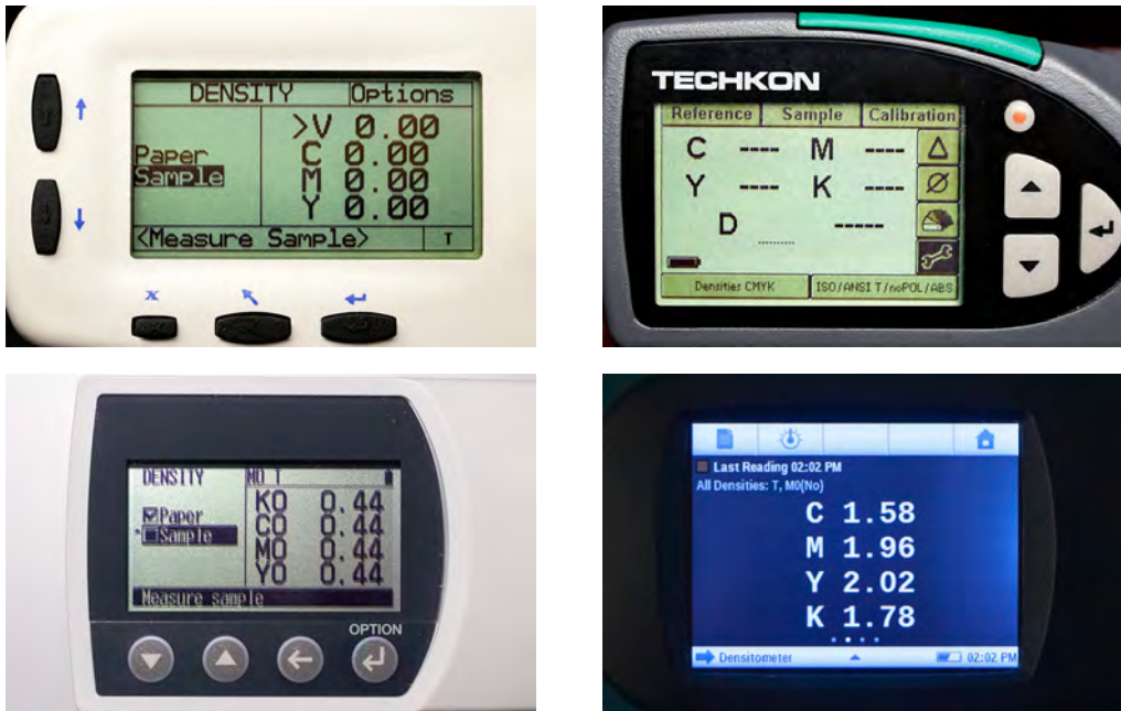
Figure C.4 "All" density display modes on X-Rite 528 (top left) Techkon Spectrodens (top right) Konica Minolta FD5 (bottom left) and X-Rite eXact (bottom right)
