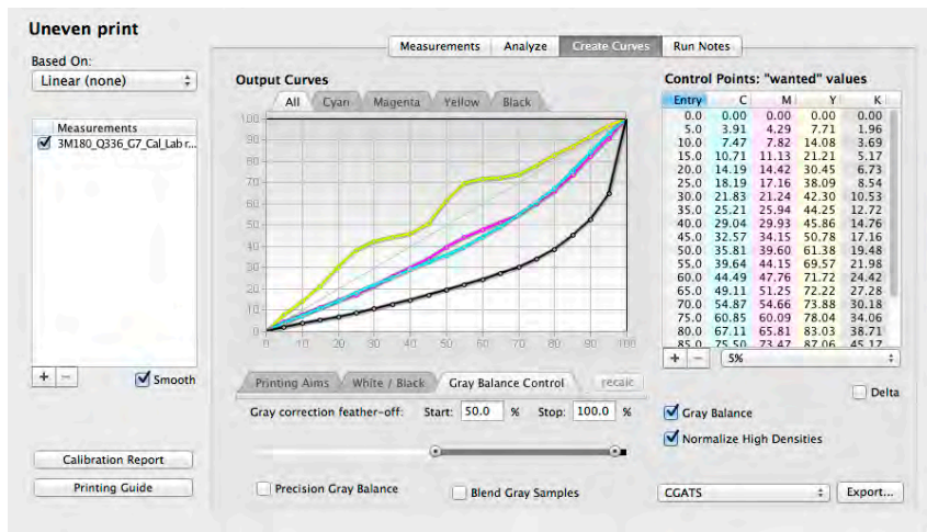
Figure 14.7 Shadow reversals eliminated by Normalize High Densities
