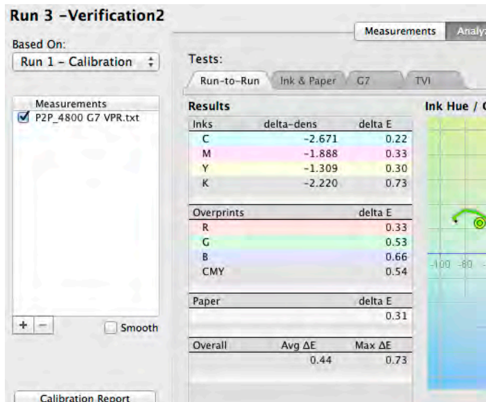
Figure 13.6 The Run-to-Run tab showing solid ink density and \Delta E variations between two runs
