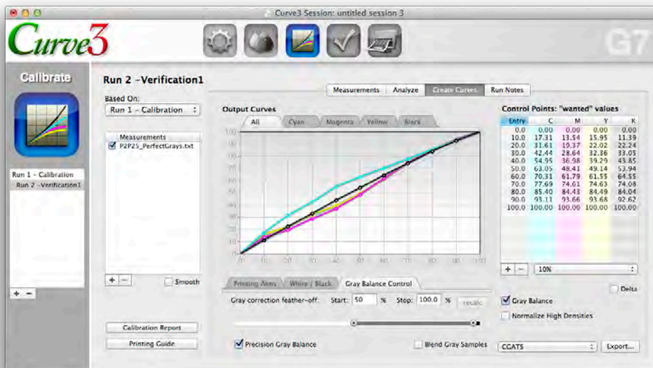
Figure 13.2 A verification Run based on Linear, showing no need for further correction
