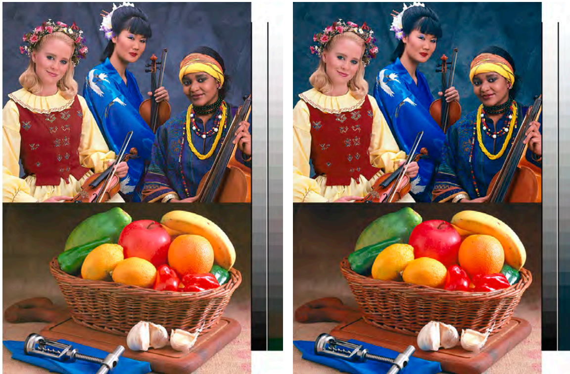
Figure 5.28 (Left): A high-density ink jet printer with conventional G7 calibration. (Right): The same printer calibrated with the Normalize High Densities option. Notice the smoother tonality in high-saturation areas (apple, garments, etc.) in the right-hand sample. Also note that the black scales are identical and the lighter half of the CMY gray scale is identical in both prints.
