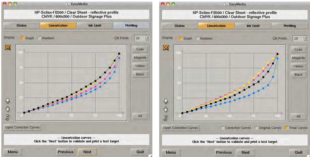
Figure 12.4 Caldera's original curves (left) and with Curve3 corrections added (right)
