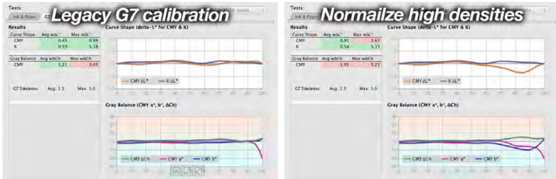
Figure 14.11 The Normalize High Densities option (right) may produce results that are theoretically further from official G7 tolerances, compared to legacy G7 calibration (left).
