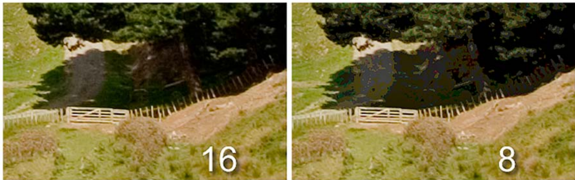
Shadow areas show unwanted “posterization” in the 8 bit image (right) compared to the smooth high-bit image (left)
