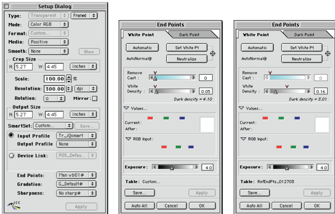
iQscan Setup dialog (left) and typical endpoints for transparency (middle) and reflection (right)
